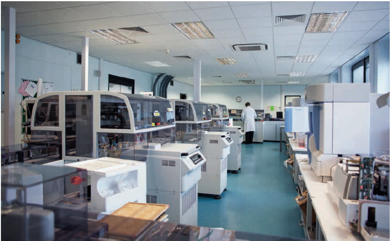
The heart of the lab is a single, oval track capable of loading more than 1,600 sample tubes per hour.
