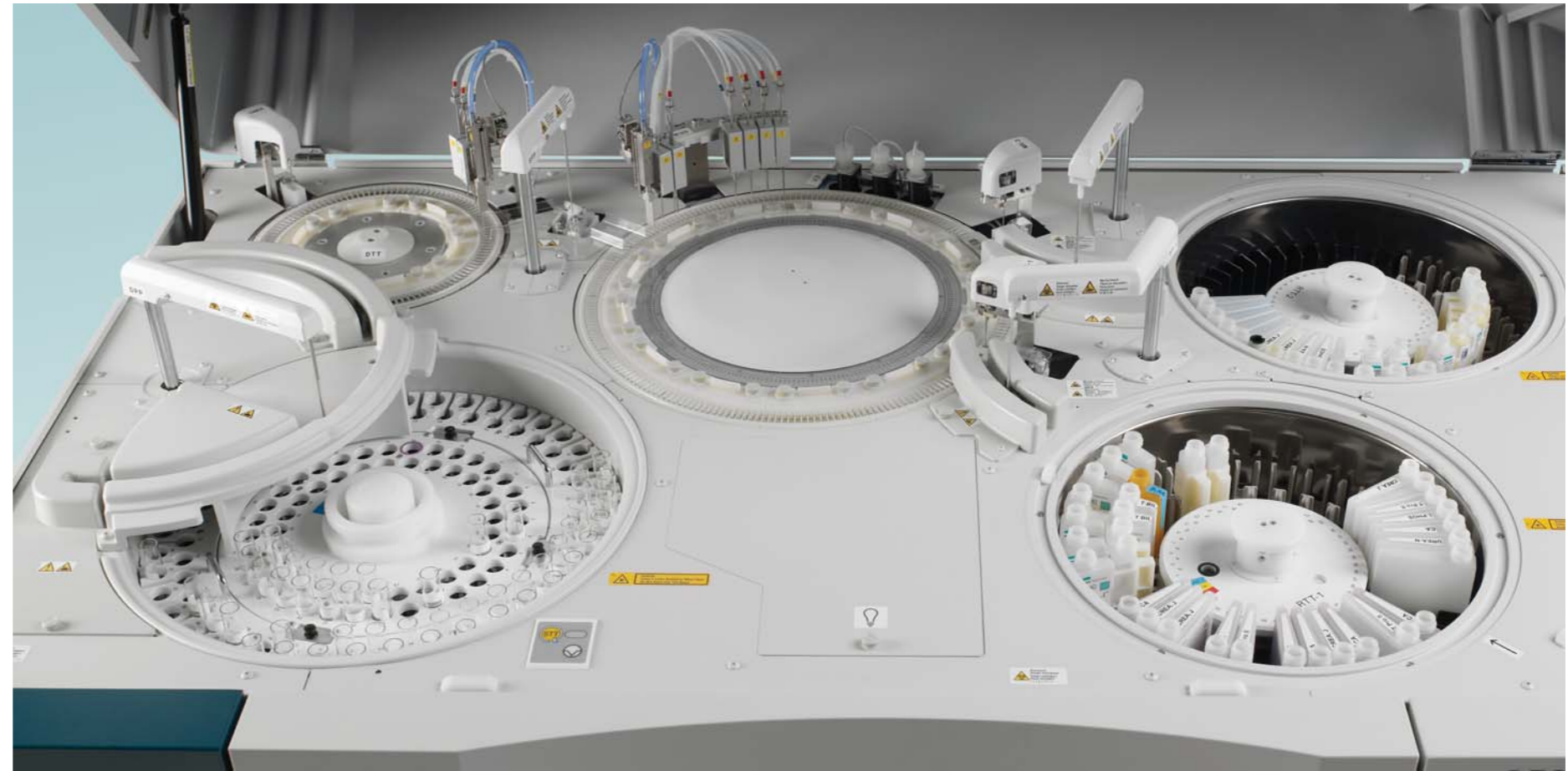
Point-in-space technology: primary probe can swing out 225° for sampling without requiring additional robotic interface
