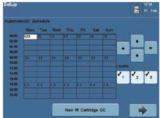
Figure 3. Siemens blood gas analyzers can be configured to meet user-defined QC schedules. Fully customizable QC schedules include selecting the day, time interval and level of QC to be run.
