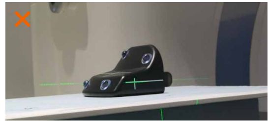
Calibration board placed on un-even foam block
