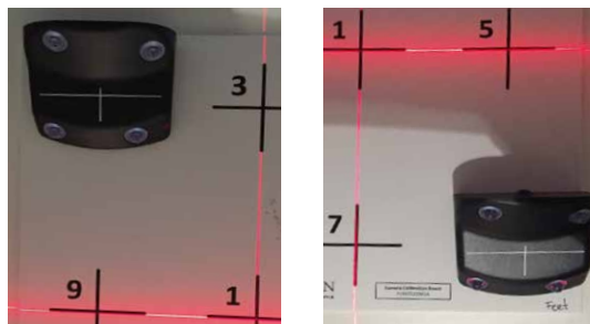
Figure 17 A, B: Example positions of marker block during calibration in case of 9 points calibration.
