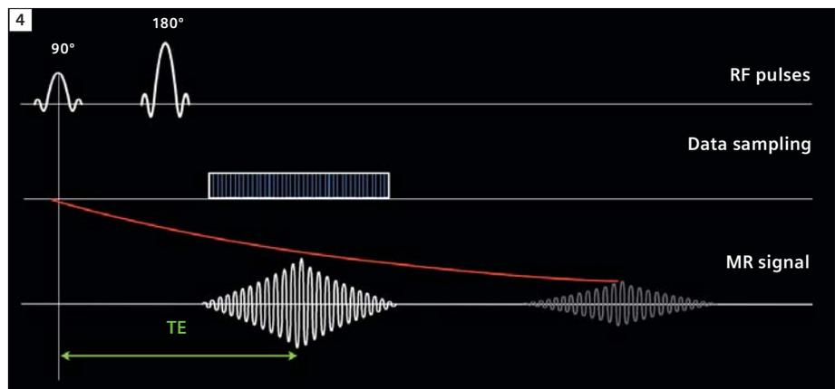
4 Benefits of faster sampling for: (I) reducing susceptibility distortions (less accumulation of phase errors), (II) reducing  $T_2^*$  blurring (faster sampling) and (III) enabling shorter TE (due to the faster sampling of  $k$ -space, which in turn brings the center of the readout window closer to the 180° pulse).
