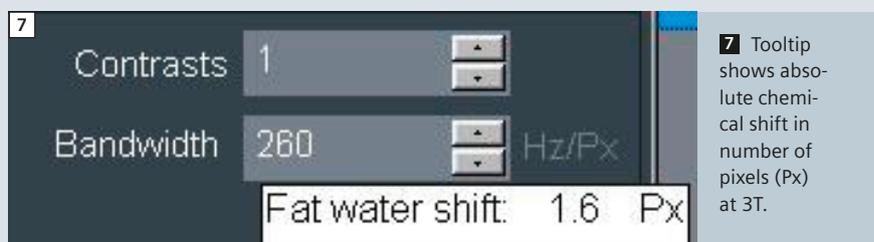
Table 2 shows the effects of optimizing a TSE protocol with respect to change of bandwidth and resolution for a 1.5T scanner. Identical SNR is the border condition for these four examples. TE was kept in the mid thirty ms range. The
