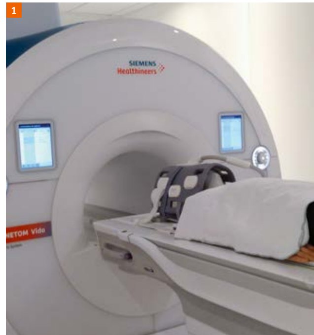
Figure 1: Patient examination in radiotherapy specific position using a flat table top, a thermoplastic mask and a flexible body coil in the MAGNETOM Vida.
