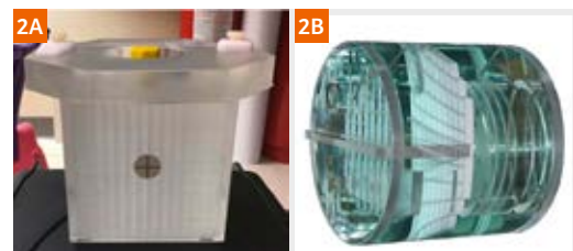
Figure 2: (2A) Quasar GRID 3D image distortion phantom (2B) Standard ACR
