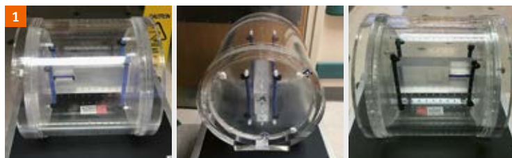
Figure 1: Quasar MRID 3D geometrical distortion phantom
