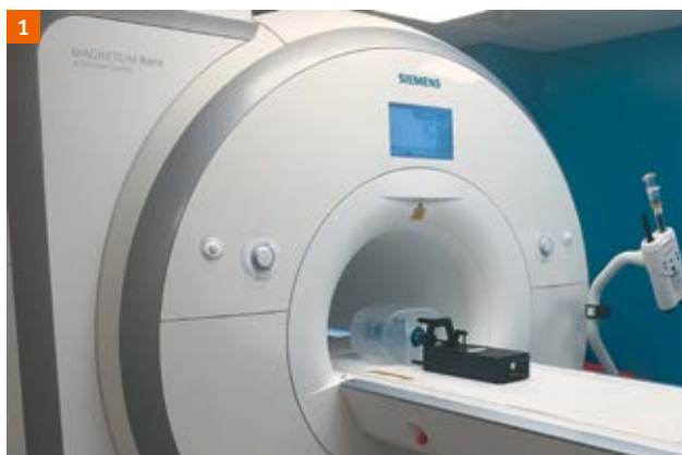
Figure 1: The Quasar™ MRI 4D motion phantom placed in the 1.5T MAGNETOM Aera bore.
