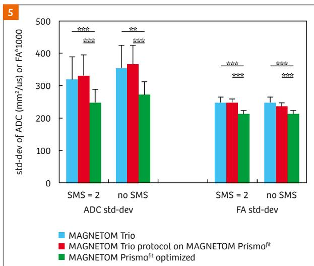
**Figure 5:** Standard-deviation of the values of ADC and FA in the segmented corpus callosum, after detailed offline processing, for the three different scan procedures described in Figures 3 and 4 on the MAGNETOM Trio and MAGNETOM Prisma<sup>fit</sup>, averaged over 8 subjects. Here, data from the SMS = 2 / 64-direction and the no SMS / 30-direction DTI protocols are shown.
