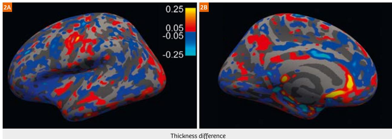
**Figure 2:** Surface plots of average cortical thickness difference for pairs of T1-weighted images acquired on the MAGNETOM Trio and the MAGNETOM Prisma<sup>fit</sup>. Thickness differences are thresholded at  $\pm 50$ – $250 \mu\text{m}$ , color bars are in mm. The left hemisphere is shown – results are similar for the right hemisphere.
