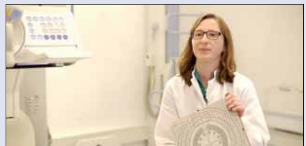
The use of a phantom enables the generation of objective data concerning image quality. The phantom used in the study at Mannheim was the Primus DL model from IBA Dosimetry GmbH in Schwarzenbruck, Germany.
